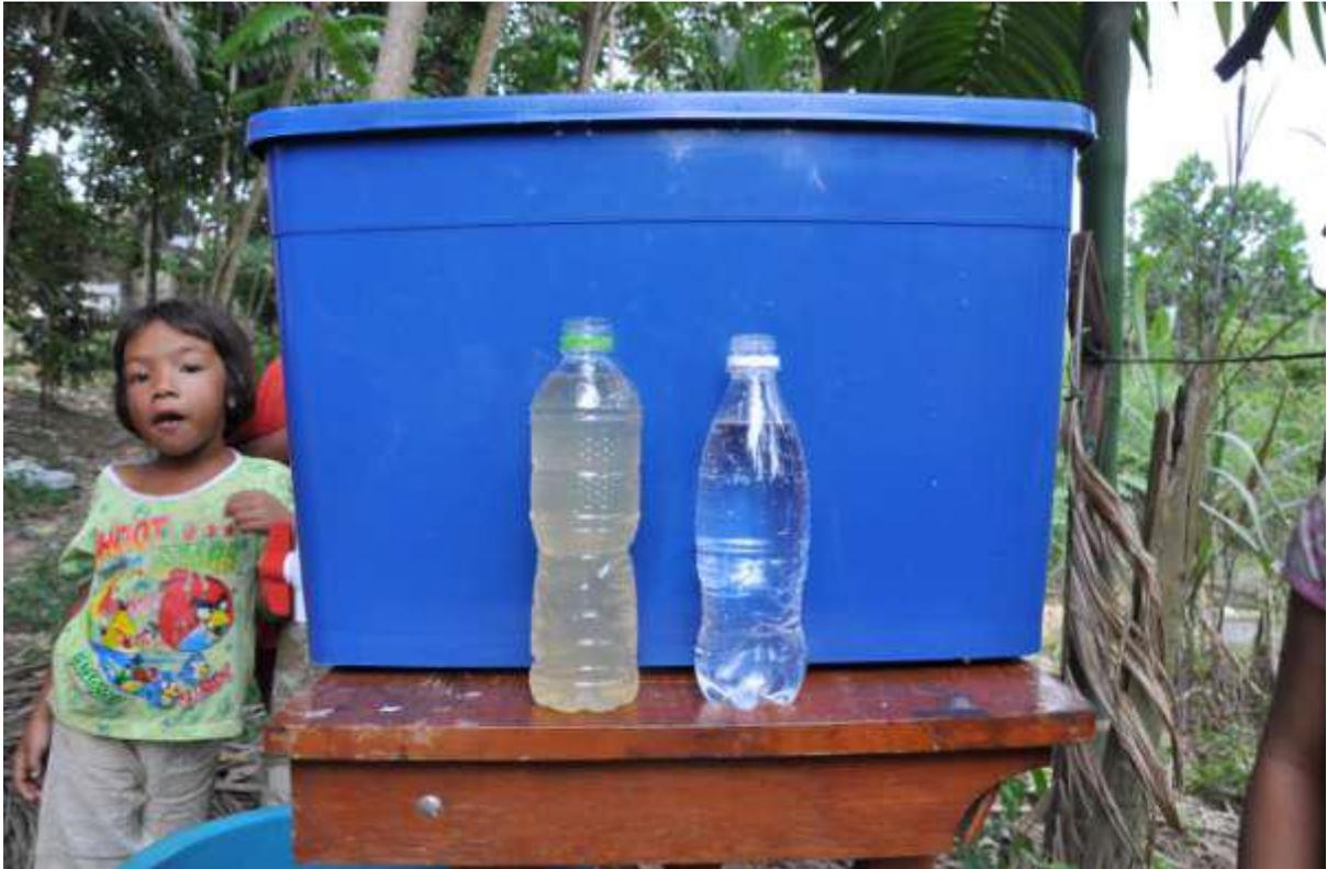
**Photo 8.0: Water comparison, pre and post SkyBox™ filtration**
